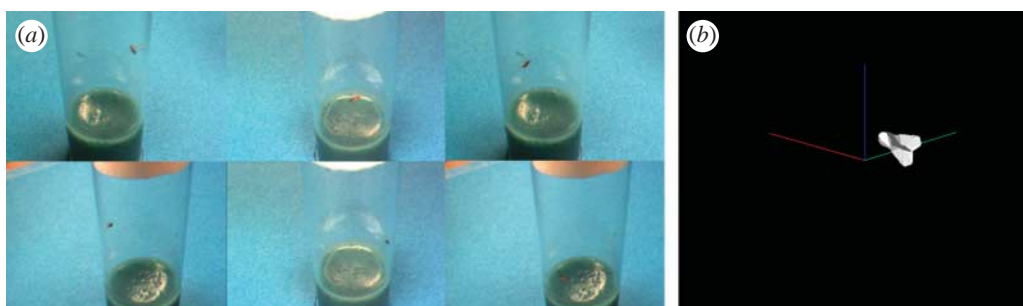
Figure 14. (a) Single fly as seen by six cameras and (b) the three-dimensional visual hull reconstruction of the fly.
